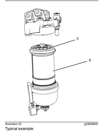
8. Rotate the filter element (5) counterclockwise and remove the filter element. Clean the filter bowl.
